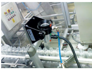
The Model 7292 Ion Air Cannon System eliminates the static and dust prior to filling the bottles.
