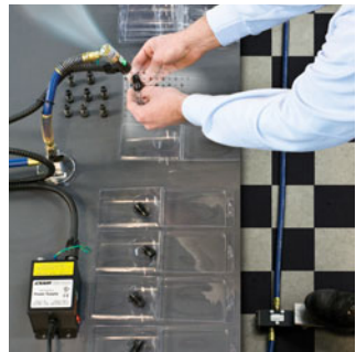
The Model 7910 Instant Static Elimination Station removes contaminants on plastic clamshell packages.
