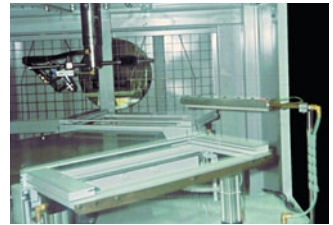
A Model 7212 12" (305mm) Standard Ion Air Knife System cleans metal frames prior to powder coating.
